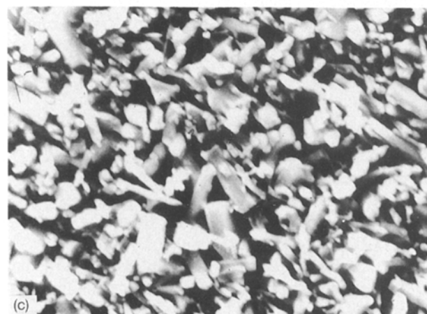
Figure 1(a-e) Scanning electron micrographs of the morphology of polycrystalline ZnO samples 1-5, respectively. \times 1500
