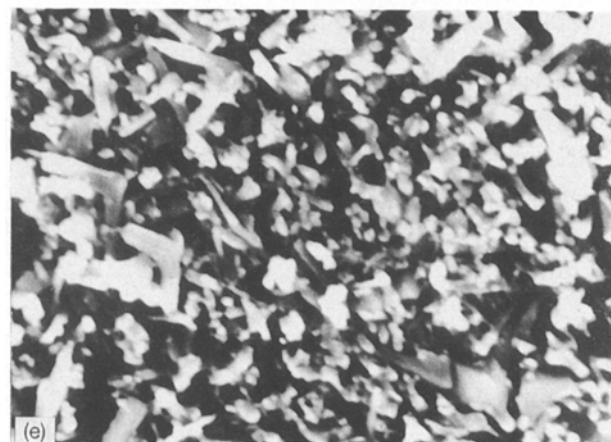
Figure 1(a-e) Scanning electron micrographs of the morphology of polycrystalline ZnO samples 1-5, respectively. \times 1500
